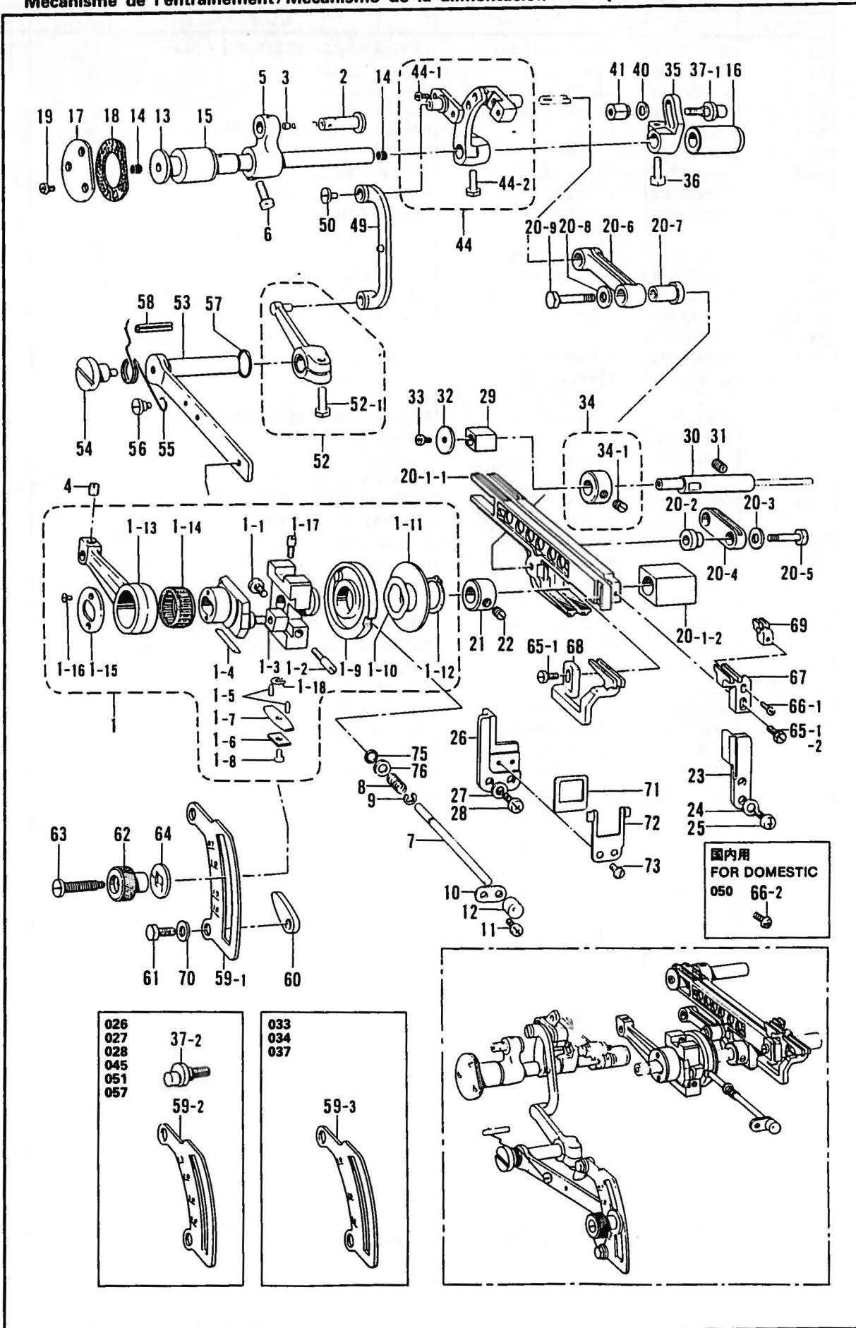
F. 送り関係/Feed mechanism/Transportvorrichtung/
